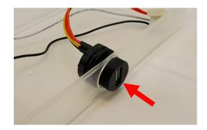
**Step 4)** Insert the USB port, flat side up, into the new 18R2 back enclosure. Then, screw on the nut and USB cap.
