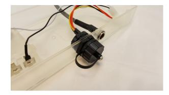
**Step 5)** Plug the battery harness and USB port harness back into 18R2.
