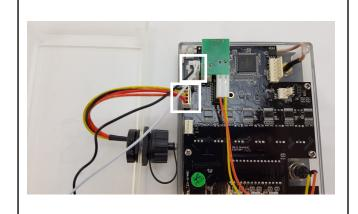
Step 3) Unscrew the USB cap and nut. Then push the USB port inward to remove it from the 18R2 back enclosure.
