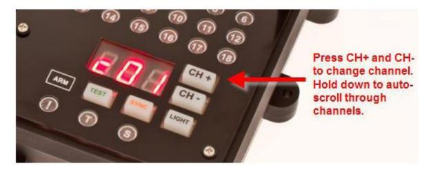
To fire the first 18 cues (cues 1-18 on channel 00), set the remote channel to 00 and fire the cues using either the manual, step or sequence firing methods (see <u>FIRING CUES</u>). To fire the remaining 18 cues (cues 1-18 on channel 01), set the remote channel to 01 and fire the cues using one of the three available firing methods. You can also step-fire and auto-sequence fire between channels (see <u>FIRING CUES</u>).
